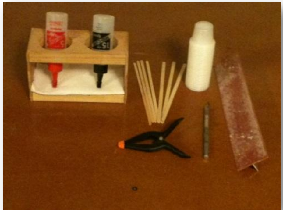
Figure 3: Custom-built rack stores epoxy upside down to minimize air and facilitate use.
