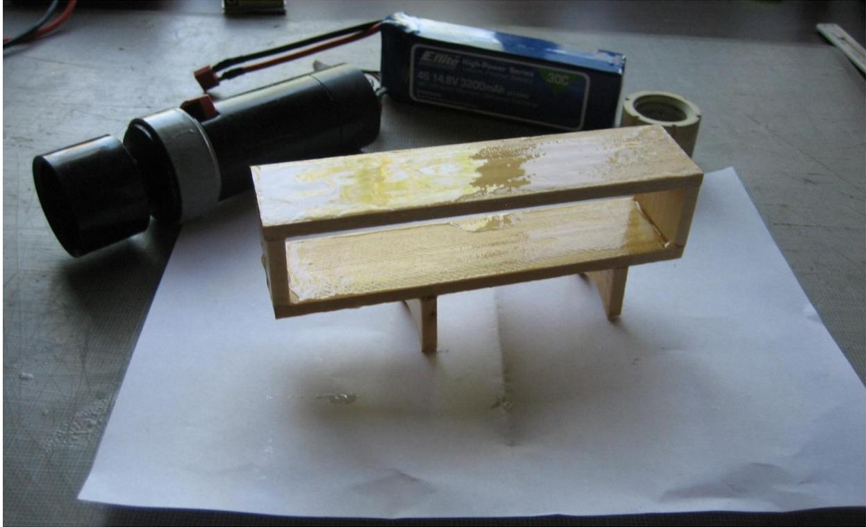
Since the unit was going to be used near glow fuel. I fuel proofed the whole assembly with the same 5 minute epoxy that I glued it together with. Additionally I found it was easier to just spread the epoxy using a gloved finger ( Yes, I know, I'm a hack ).
