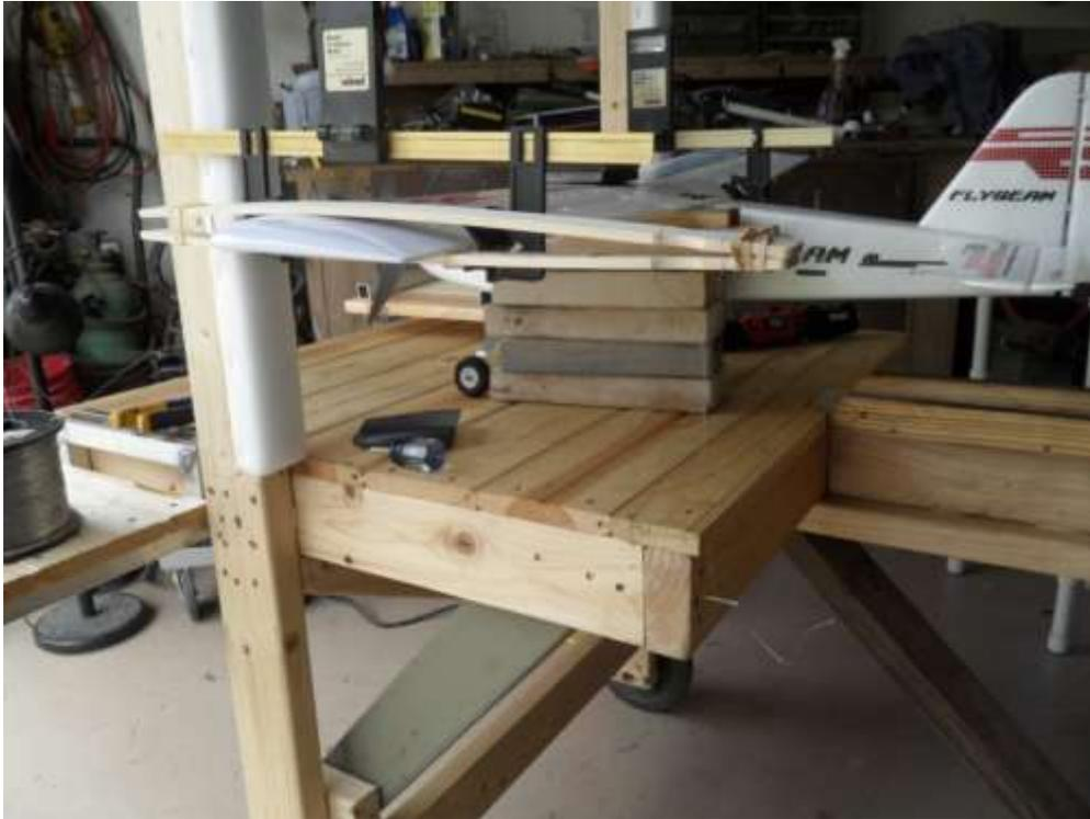
While the water is getting hot check the twist with Robert Incidence Meters. Using paint sticks and rubber bands (or some other materials you have available) affix a lever to the wing. The root of the wing is secured with blocks and a weight (not shown). The wing tip is twisted slightly more than required as there will be some resistance to the twist force. In this case a tip support/fulcrum opposite the twist wasn't required. On longer wings it probably would be to keep the wing from curving.
